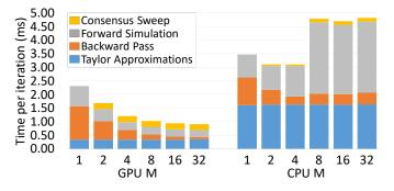
These tradeoffs led to the GPU outperforming the CPU across parallelization options
